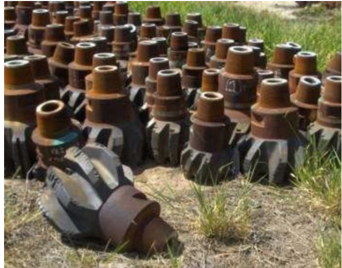
Figure 4-4: Fixed Cutter Drilling Bits
