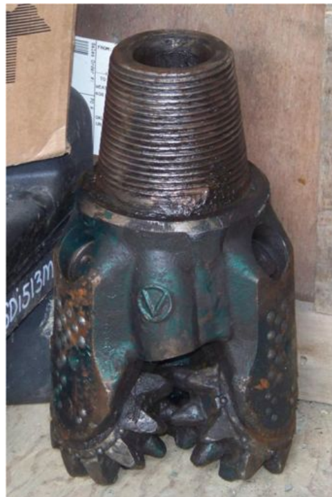
Figure 4-5: Example of Tricone Rotary Drill Bit
