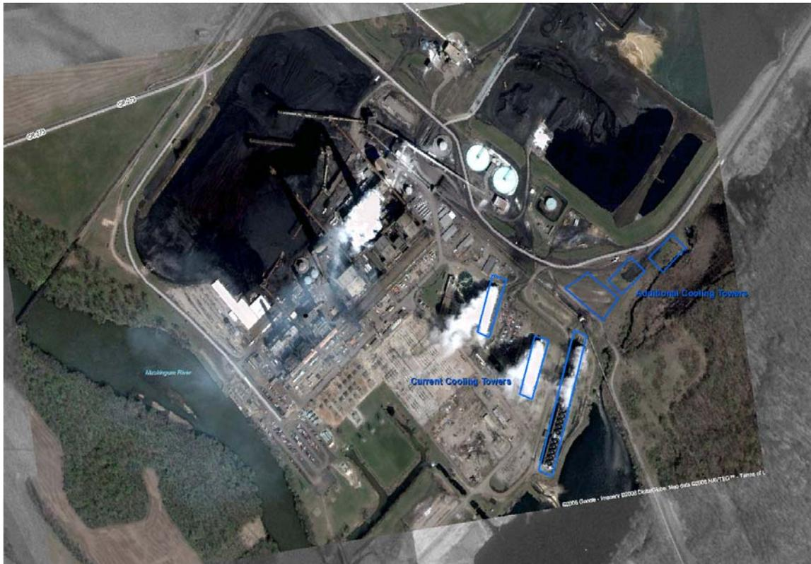
**Figure 1-14. Current and Additional Recirculating Cooling Required to Retrofit All Units with 90% CO<sub>2</sub> Capture and Compression at the Conesville Plant**
