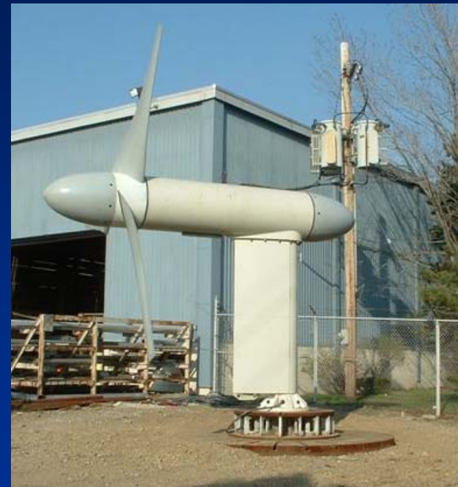
35 kW turbine with downstream rotor, 5-m in diameter, which yaws to accommodate reversing flow
