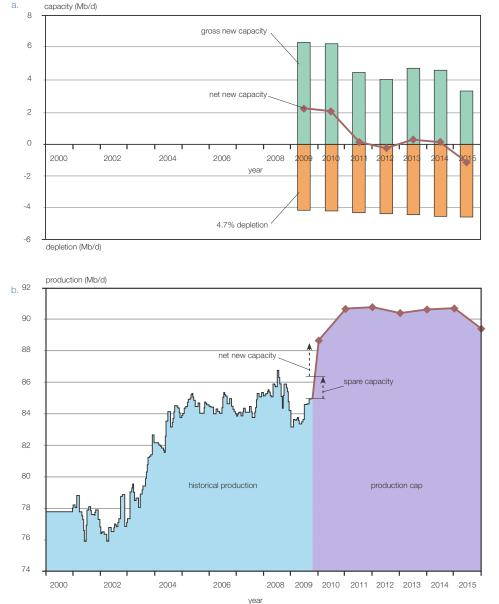
Fig 3.2 Derivation of the maximum future production capacity or "production cap".
