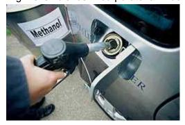
similarly to E-85 in flex fuel vehicles, M-85 and even neat methanol, or M-100. Displacing gasoline on an energy basis is a greater challenge given methanol's lower energy content. If using mixes above M-70, separate considerations would need to be made for materials compatibility and an upgraded fuel pump and fuel sensor may be necessary for some vehicles, which could raise the incremental cost of vehicles by up to \$490.
