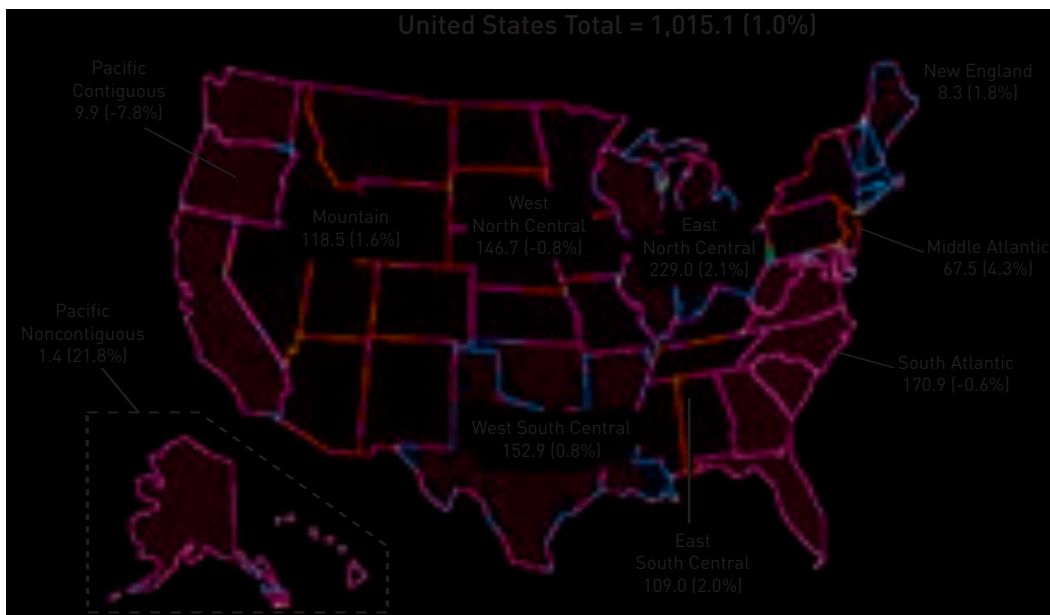
Figure A.9.1 Electric power-sector consumption of coal by Census region, 2004 (million short tons and percent change from 2003) (EIA, 2005).
