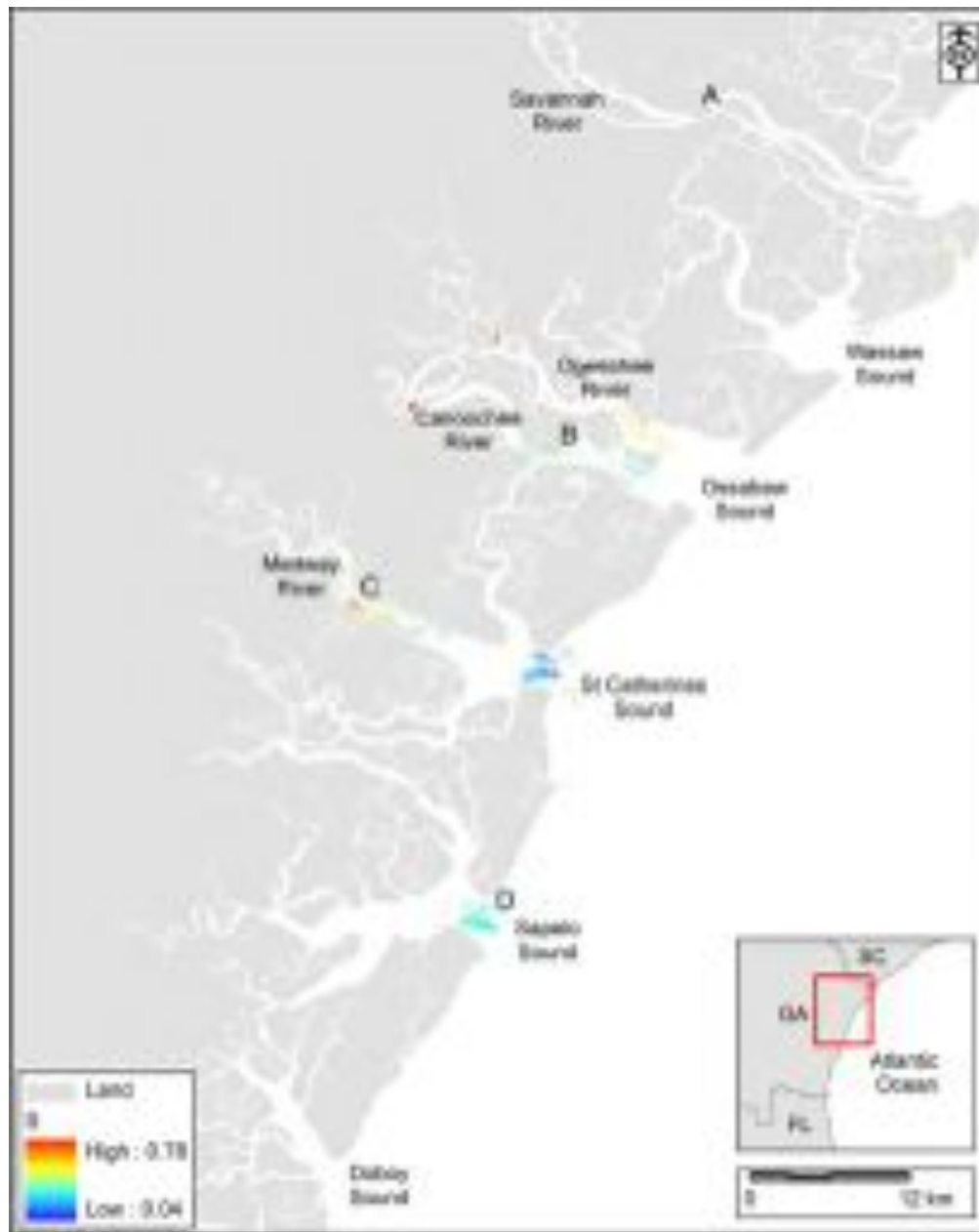
Fig. 7. Candidate locations with tidal power conversion potential on the northern Georgia coast that are determined by applying the site selection methodology.
