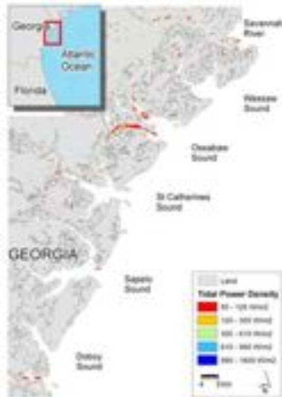
Figure 10. The effective power density using depth filter h_{min} = 7 m, the efficiency curve in Figure 7 and a minimum power density of 50 W/m 2 for the northern Georgia coast.
