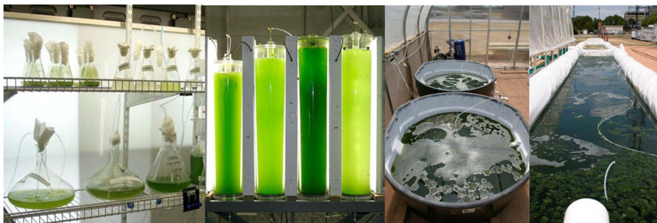
Fig. 3 Algae were grown in four growth stages: 1) flasks 2) seven indoor photobioreactors (L1 – L4 shown, ~100 L each) 3) four greenhouse tanks (G1 and G2 shown, ~1000 L each) and 4) two covered outdoor ponds (shown without the cover, ~2400 L each)
