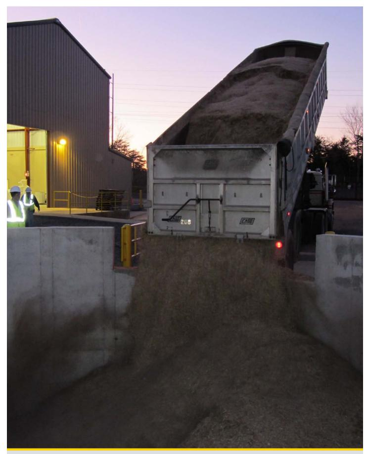
After passing through the forage harvester, low-moisture switchgrass becomes a free-flowing bulk material that can be easily dumped into the receiving pit. Properly timed use of the forage harvester yields better particle size distribution and bulk flow than tub grinding of baled switchgrass. *Photo: Al Womac*
