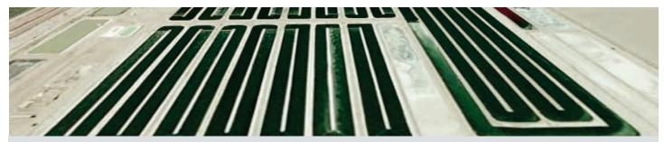
Algae are often grown in outdoor raceway ponds to ensure adequate exposure to sunlight. Research suggests biofuels from microalgae alone could displace 17% of today's transportation fuel imports. *Photo: PNNL*
