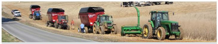
A pull-type forage harvester, tip wagons, and trucks stand ready for harvest at the edge of a switchgrass field. The harvester (scalable for commercial use) creates the bulk format, and the tip wagons and trucks collect the loose bulk format for transport to near-by storage. Bulk compaction increases the density of low-moisture switchgrass for transport over longer distances. *Photo: Al Womac*
