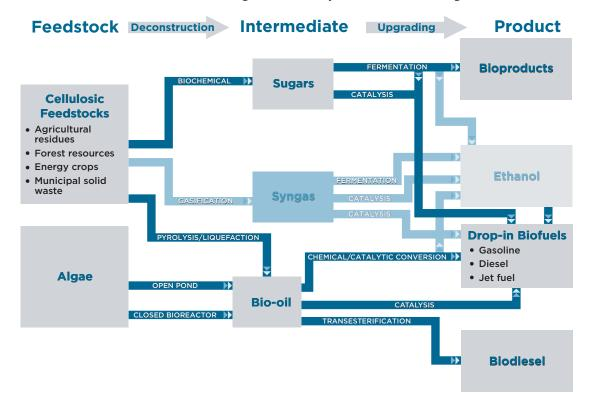
The Biomass Program is concentrating high-value, high-risk RD&D on the key conversion pathways for deconstructing biomass into sugars and bio-oils and then upgrading those intermediates into advanced hydrocarbon fuels. *Illustration from Energetics Incorporated*
