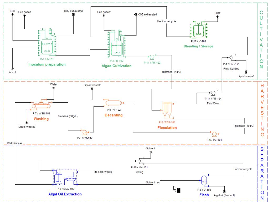
Figure 2:  $\text{CO}_2$  photobiocapture pilot technology flowsheet
