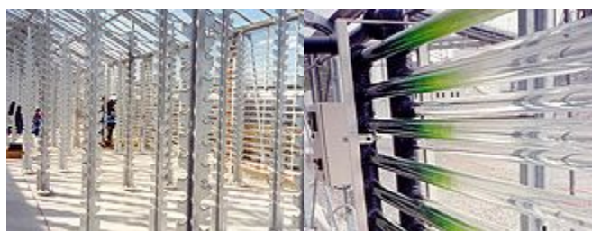
FIGURE 2-7 Tubular photobioreactors of straight horizontal tubes stacked in vertical fence-like arrays housed in a greenhouse in Klotze, Germany. SOURCE: Algomed. Reprinted with permission from AGU.
