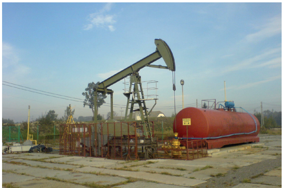
Figure 4 The well in Kaniów that was used as CO 2 injection well and that is used as production well in the MOVECBM project.
