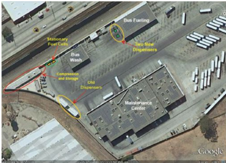
Fig. 6. The Oakland, CA, fueling station of AC Transit capable of dispensing 360 kg/day.
