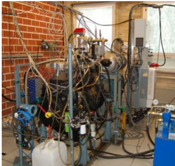
Figure 2. LEO research engine used in the ReFuel high-speed engine runs.
