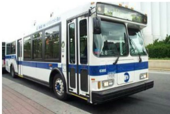
Figure 6: Orion VII bus with BAE Systems HybriDrive hybrid propulsion system.
