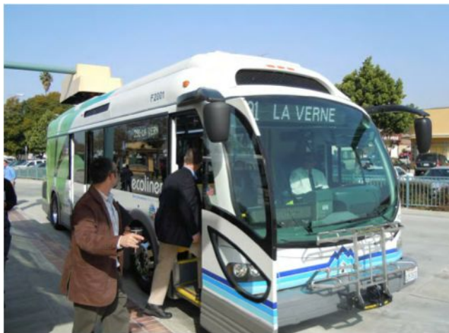
Figure 12: Proterra electric bus in Foothill Transit with super-fast charging at bus stop (photo courtesy of Veolia Environnement)
