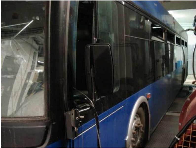
Figure 8.3. A test bus on Environment Canada's chassis dynamometer.
