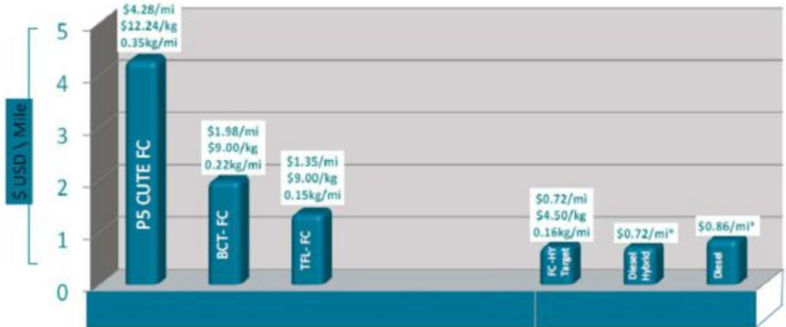
Fig. 5. Fuel costs for fuel cell and diesel/diesel-hybrid transit buses. To become competitive with conventional transit buses will require improvements in fuel cell efficiency and hybridization strategies, and a considerable reduction in the cost of H 2 .
