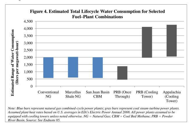
at an NGCC power plant. Thus, the type of cooling system employed plays an important role in determining the overall water implications of choosing to generate electricity from coal or natural gas.
