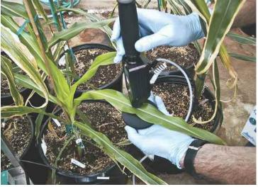
Advances in technology can help improve current biofuels and develop new alternatives. This near-infrared spectrometer, promoted by the National Renewable Energy Laboratory, enables researchers to chemically analyze plants and trees in the field, increasing the speed of the analysis and cutting down costs.
