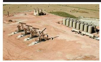
Fig. 3. Producing wells on one of the 40 ECO-Pad drilling locations that Continental Resources intends to have in operation by the end of this year. Continental credits the technique with reducing costs as much as 10% per well. Courtesy of Continental Resources Inc.
