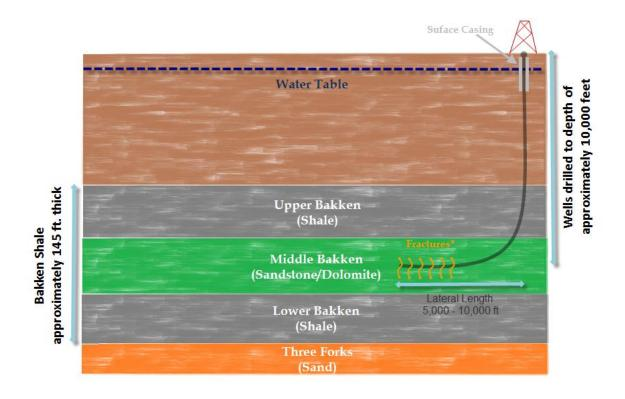
Figure 2. Example of Horizontal Drilling in the Bakken
