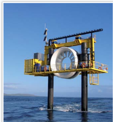
An open-ring turbine prototype being tested in Europe.
