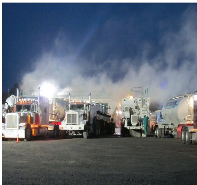
PICTURE 2. TRUCKS HOT LOADING WATER MIXTURE AT A FRACKING SITE
