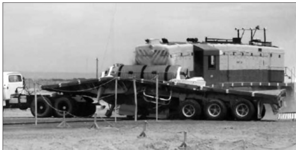
FIGURE 10 Spent fuel crash test performed in 1977. A locomotive traveling at approximately 80 miles per hour crashed broadside into a used fuel transportation cask. The cask and the dummy fuel inside it performed in accordance with regulatory requirements. Source: http://www.sandia.gov/recordsmgmt/ctb1.html .
