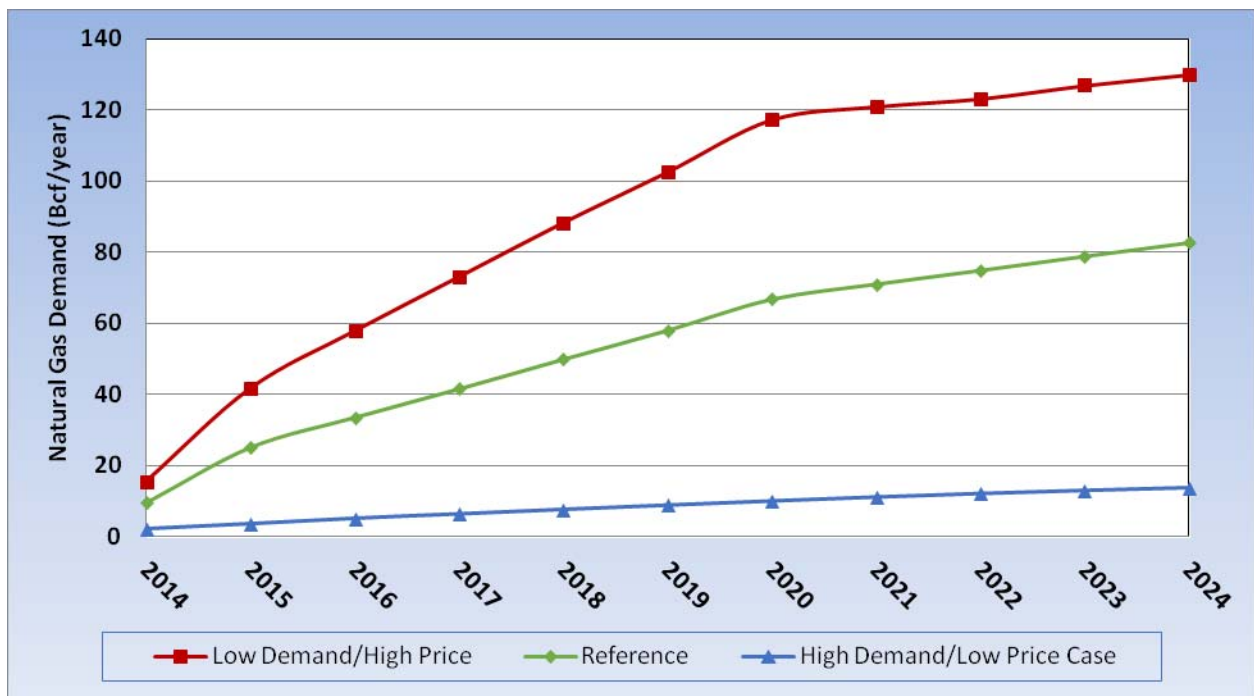
Figure 17: Natural Gas Demand for New CHP to Generate Electricity for California’s Industrial Sector Customers
