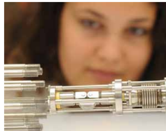
Miniaturised device for rig stress corrosion cracking tests in Light Water Reactor environments.
