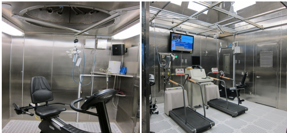
A small chamber (36 square feet) used for diesel studies (left) and a large chamber (300 square feet) used for ozone studies (right). (EPA OIG photos)
