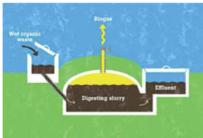
Figure 2: Basic components of a fixed-dome biogas digester plant Source: Ejigu (2010, p. 3)
