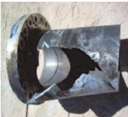
Figure 12 Metallurgical failure caused by liquid mercury
