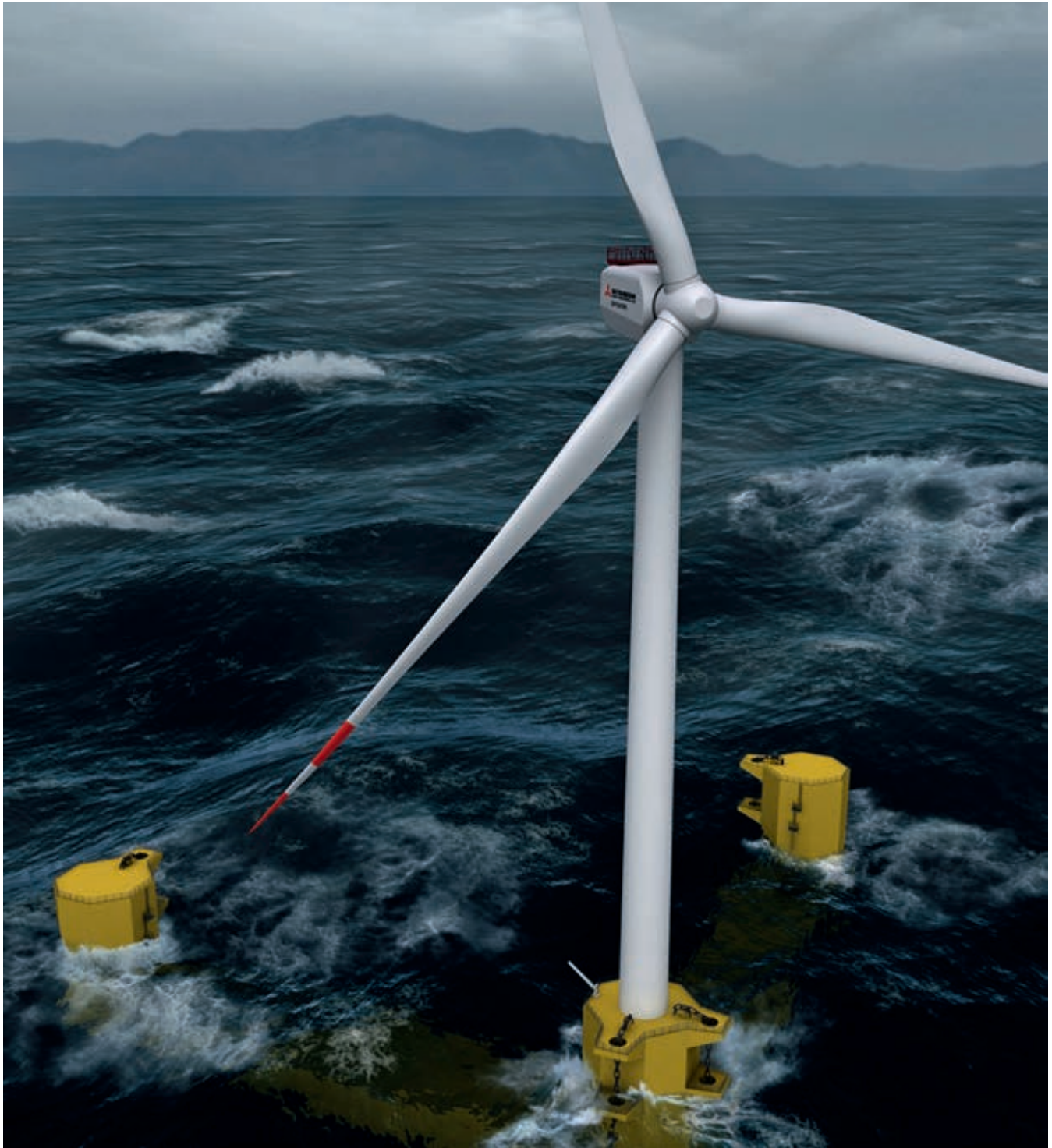
V-Shape semi-sub floater prototype with 7 MW turbine © Mitsubishi Heavy Industries, Ltd
