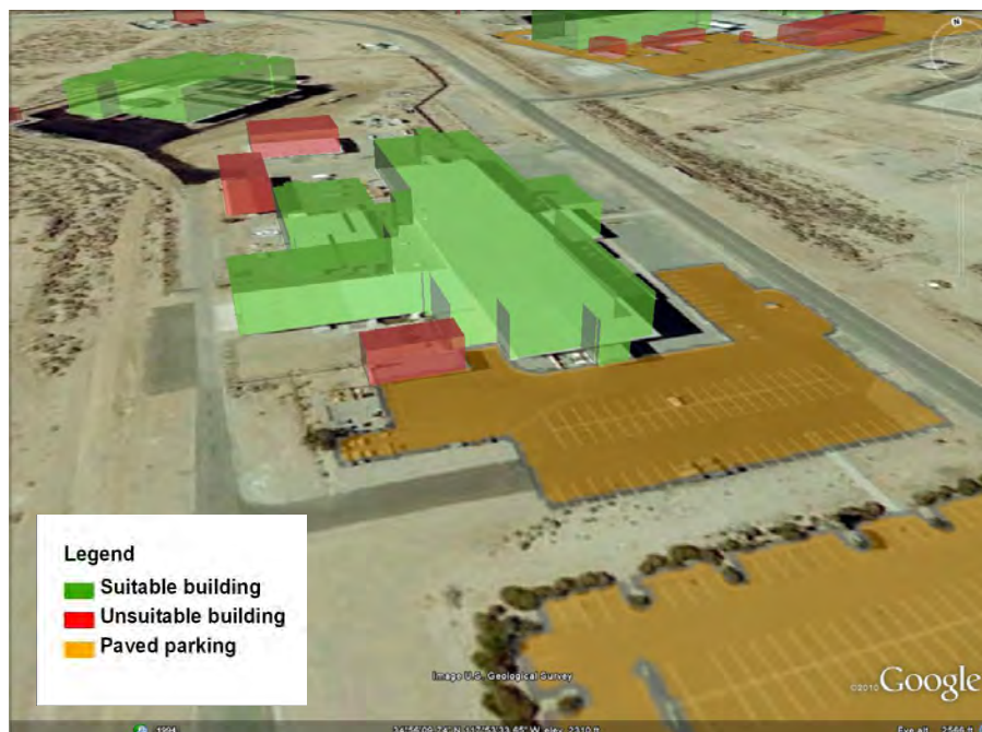
Figure 5.6 – Visual Inspection of Rooftops and Parking Areas at Edwards AFB in Tools such as Google Earth Provides Information not Available in GIS Data
