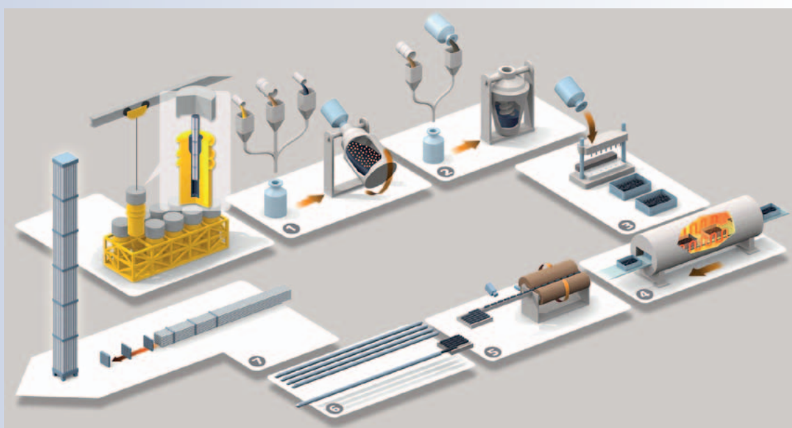
Figure 8: MOX fuel fabrication
