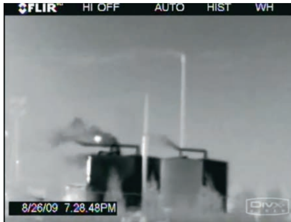
Methane released at these storage tanks is invisible to the naked eye, but it can be seen with an infrared camera.
