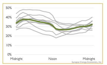
Figure 6. Hourly wind capacity factors from individual turbines versus aggregate over entire PJM region
