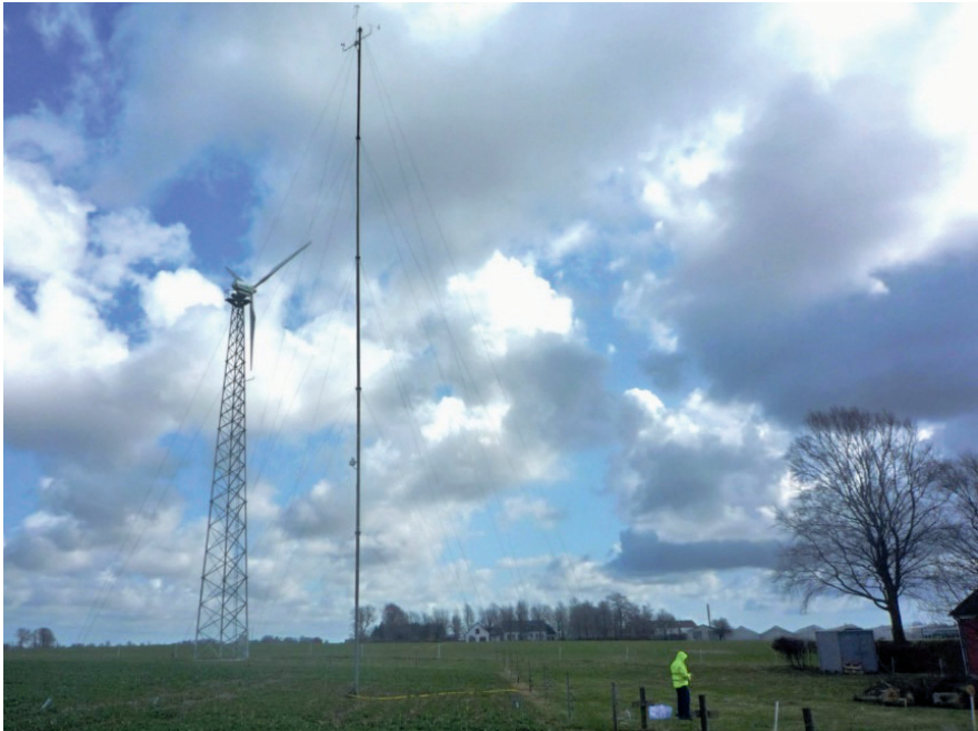
Figure 11: A WindEn 45 turbine undergoes testing by Intertek
