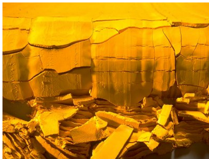
Figure 2-4: Uranium oxide concentrate ( U_3O_8 ) (Source: World nuclear news [13])
