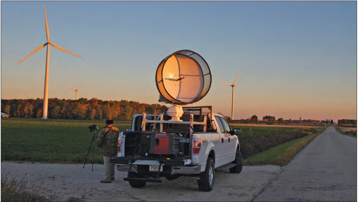
Portable radar is used to track bird flight near wind turbines.
