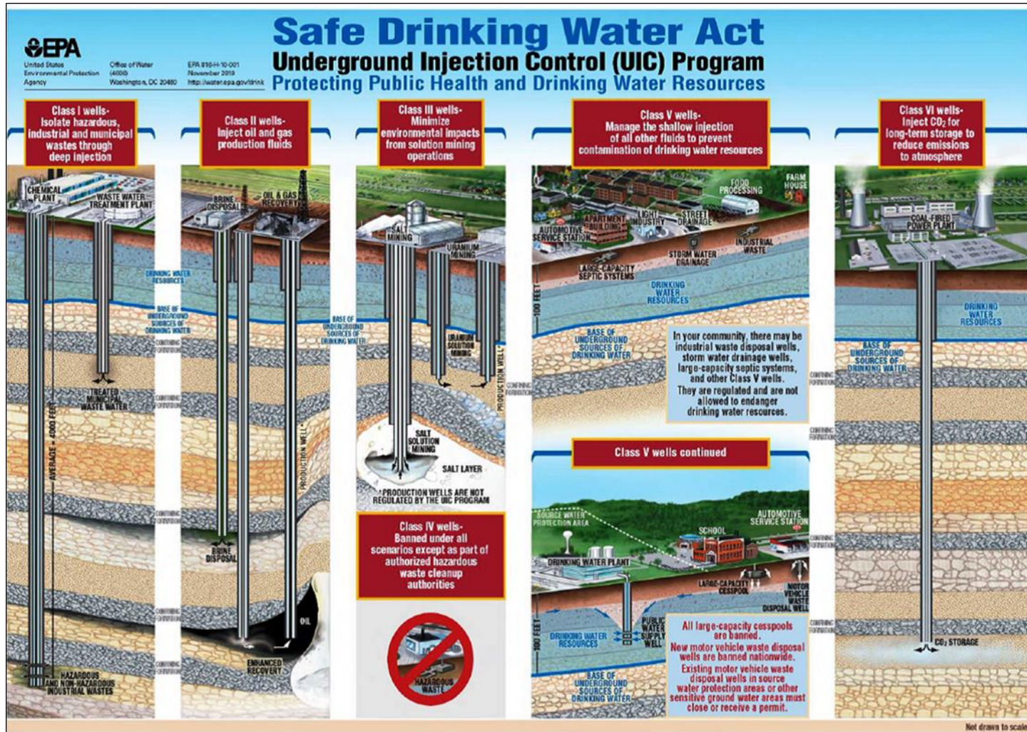
Figure 5. Federally Regulated Underground Injection Wells
