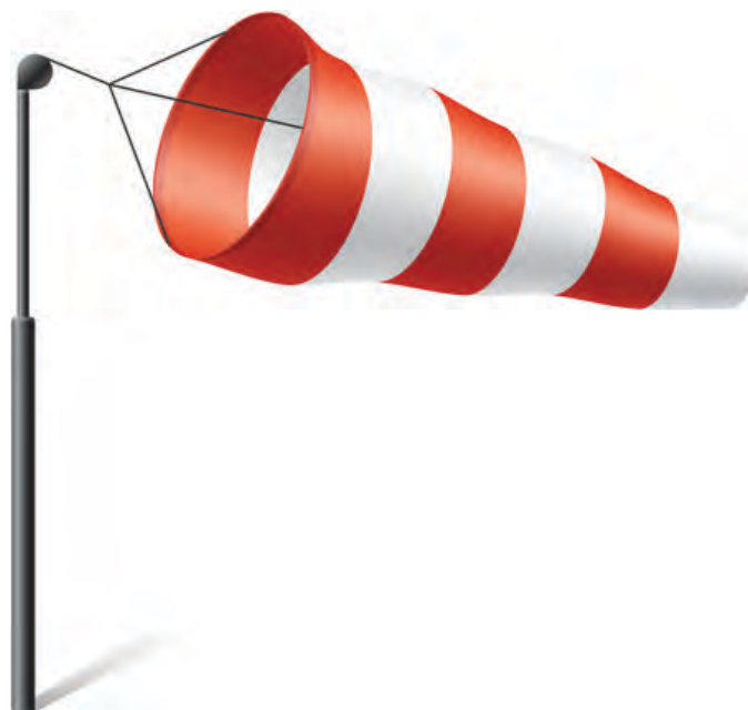
Figure 3-2. Wind sock seen at airports.
