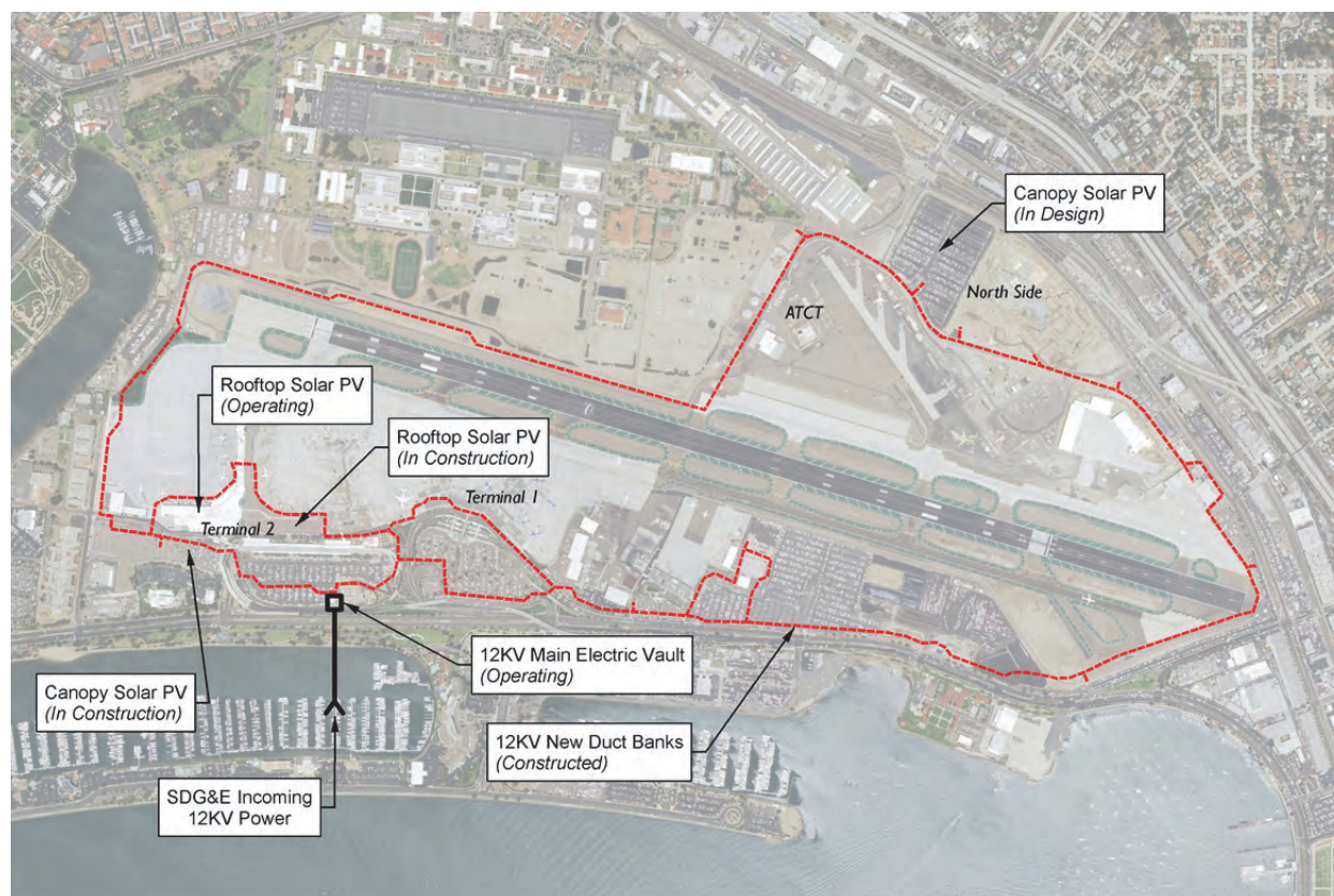
Figure 1-6. San Diego Airport microgrid.
