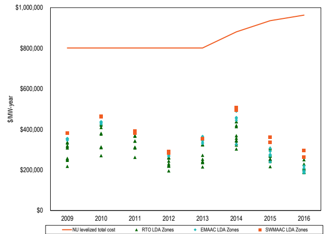
Figure 14 New entrant NU net revenue and 20-year levelized total cost by LDA (Dollars per installed MW-year): 2009 through 2016
