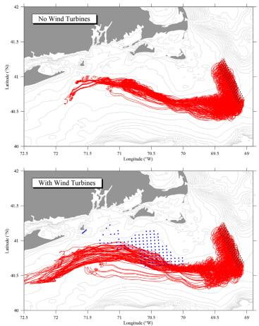
Model-predicted trajectories of particles for the cases without (upper) and with (lower) wind turbines. A total of 100 particles (black dots) were released with separate scales of 1.4 km in the east-west direction and 3.2 km in the south-north direction over the western slope offshore New England.
