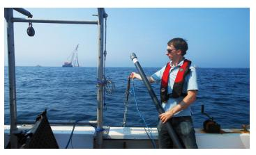
Deploying an acoustic monitor near the Block Island Wind Farm during the RODEO study.
