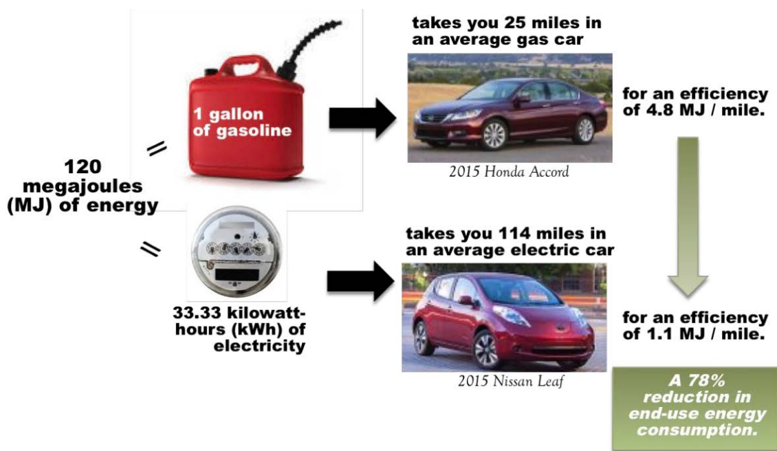
Figure ES-1: An Illustration of Relative Efficiency of EV and Gas-Fired Vehicle 1
