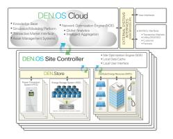
Demand Energy's Distributed Energy Network Optimization System (DEN.OS), based on patent-pending control and economic optimization technology, maximizes the economic returns of behind-the-meter storage systems alone, or in combination with distributed generation. The DEN.OS platform was architected to facilitate the design, integration and operation of energy assets/ services, providing users with
