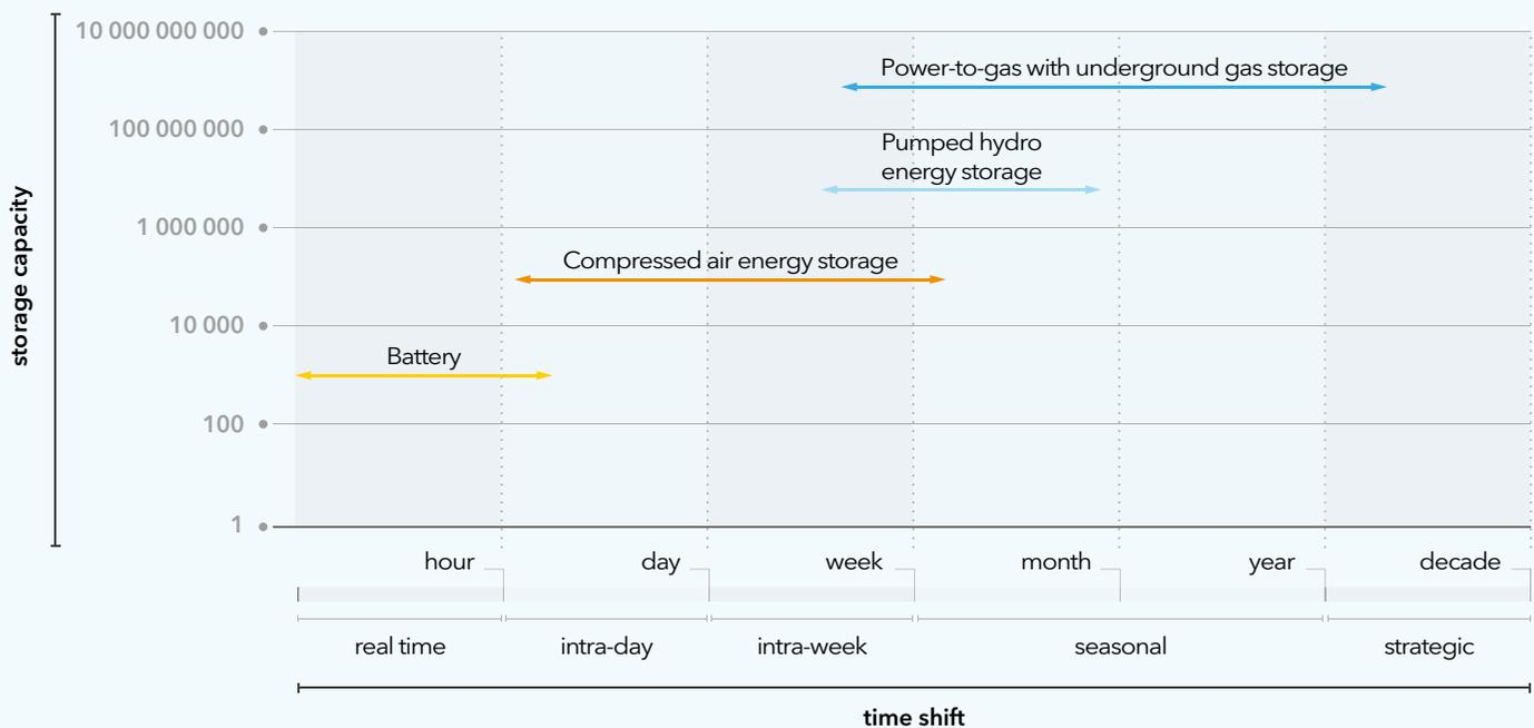
In principle, storage could be achieved by the traditional, larger-scale, solutions such as PHES and, in the future, compressed air storage units. However, neither option currently suffices for currently fast-growing surplus electricity.
