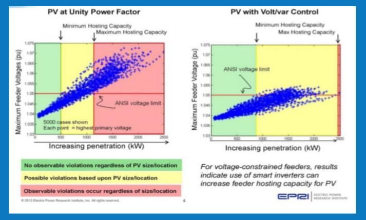
Figure 2: Improving Hosting Capacity Through Inverters (Volt/VAR control)<sup>5</sup>
