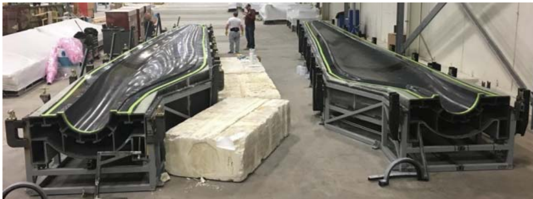
Figure 33: Additively manufactured molds ready for use, Source: ORNL
