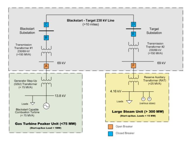
This example illustrates a situation where the blackstart generating unit (Gas Turbine Peaker Unit), cranking path and next start unit (Large Steam Unit) are owned and/or operated by different entities. As a result, significant coordination and cooperation is necessary to plan for, and perform the test. These activities are managed by the transmission operator, which has direct control over the cranking path.
