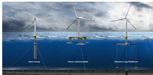
Figure 26 Different types of floating foundations.
