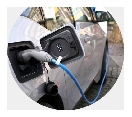
As Pod-Point highlight, a 3.7kw charger (similar in strength to a three-pin socket) takes an hour to charge 15 miles' worth of journey. A 7kw charger will produce 30 miles' worth of charge in that exact same time.
