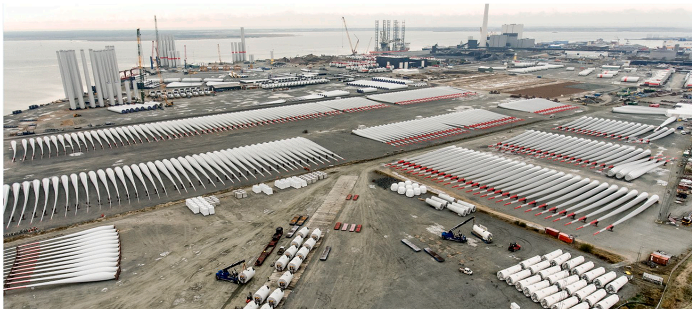
Fig. 1. An example OSW marshaling port, the Port of Esbjerg in Denmark (2017). Blades and some tower sections are in foreground, and tower assembly can be seen in background adjacent to the load out areas. For scale, the blades pictured are 80 m long. (Reprinted with permission of the Port of Esbjerg).
